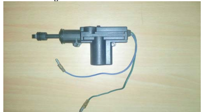
Fig -2: Electromagnetic lock
